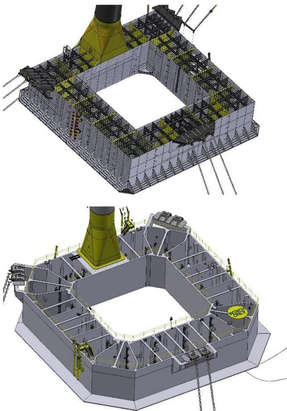
Figure 2. View of structure for 6MW floaters: steel (top) and concrete (bottom)
