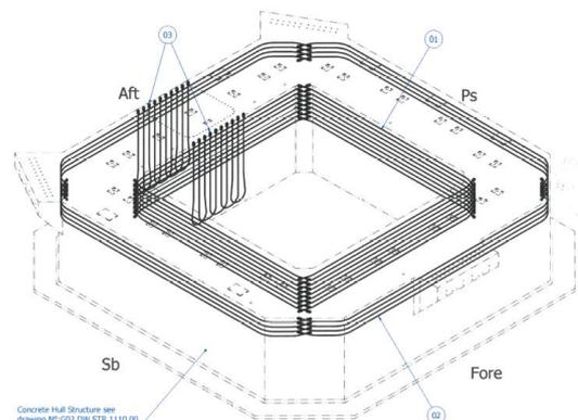
Figure 3. View of pre-stressing cables in a typical floating wind turbine
