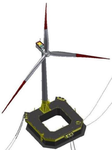
Figure 1. View of 6MW damping pool
